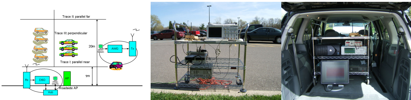
Fig.1 The diagram of a WAVE testbed and the measurement scenario (left). The pictures of an RSU (middle) and an OBU (right)
